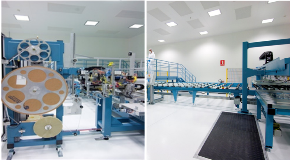
Figure 1.26: Buss tool picture (left) and clean room to handle the PVB (right).
