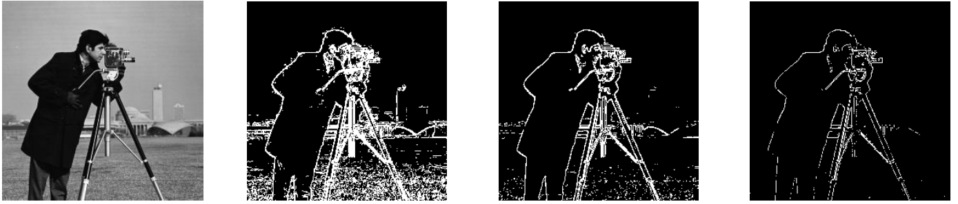
Fig. 2: Numerical simulations of our edge detection algorithm applied to the original grayscale image shown with increasing threshold T_{TH} values.
