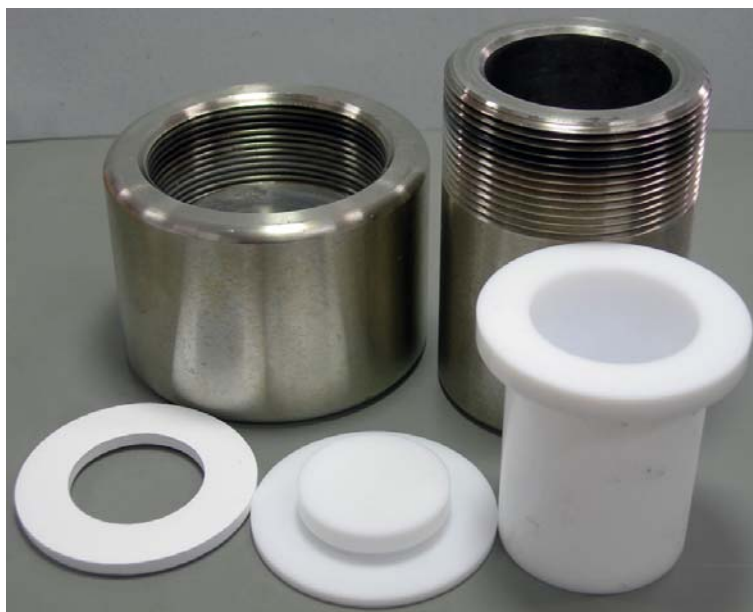
Fig. 5.1. A hydrothermal setup: stainless steel autoclave, a low-density porous polytetrafluoroethylene (PTFE) hyper-sheet ® gasket (GORE-TEX ® ), as well as PTFE cover and cell.
