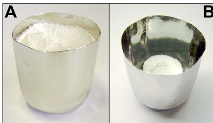
Fig. 4.1. Images of the platinum crucible before (A) and after (B) a high temperature solid-state reaction of TTCP synthesis showing the shrinkage of the precursors' mixture.
