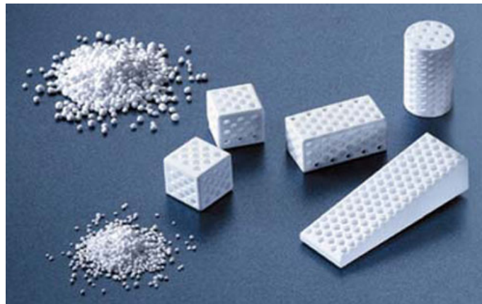
Fig. 2.17. Examples of calcium orthophosphate-based bone substitution materials (granules and scaffolds) (after Dorozhkin). 12
