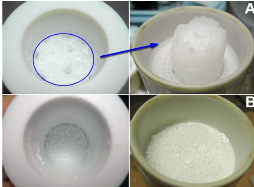
Fig. 5.3. Photo of two types of hydrothermal synthesis products: an abundant cotton-like suspension (A) and secondary wall-product (B).
