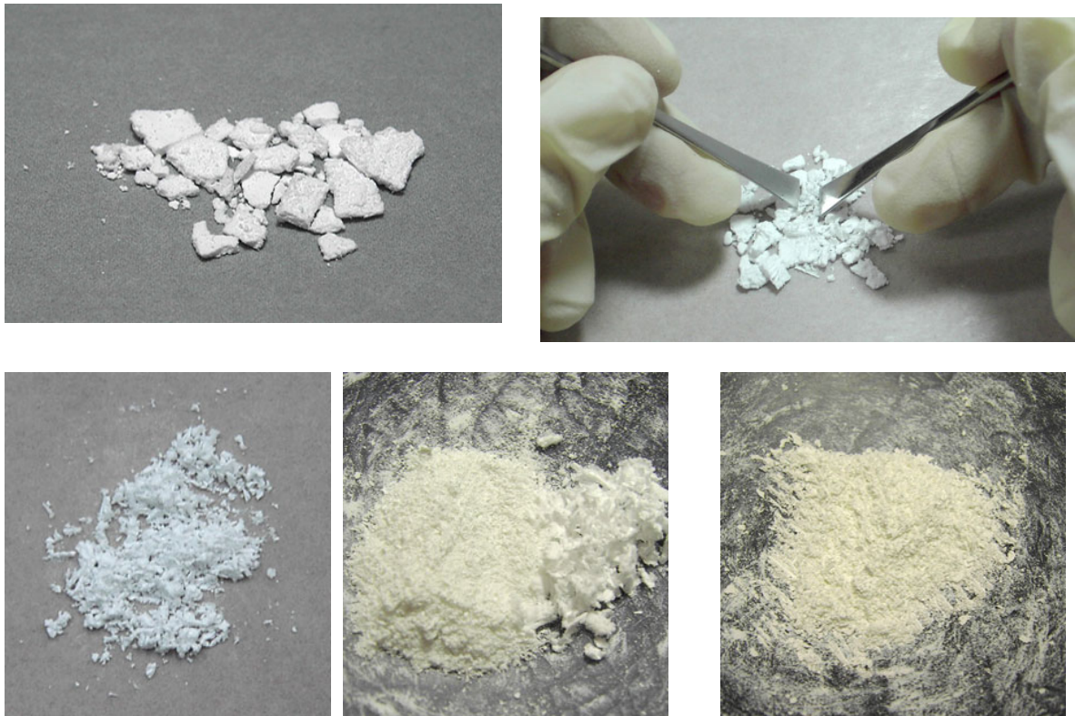
Fig. 6.1. The hydrothermally-derived HA powdered product (top left panel), the reinforcement phase during and after hand spatula dispersing (top right and bottom left panels, respectively), the reinforcement phase and the CPC precursors (TTCP and DCPD) at the agate mortar (bottom central panel), and the resulting fine powders mixture after gentle grinding.
