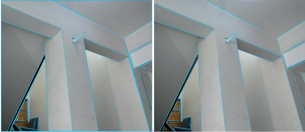
Figure 4.10: Line extraction results for the images in the dataset lowtextureI [74]. On the left, the result of LS with 194 lines extracted and cost of 0,7s. On the right, the result of SALM featuring 56 segments and obtained in 3.8s.
