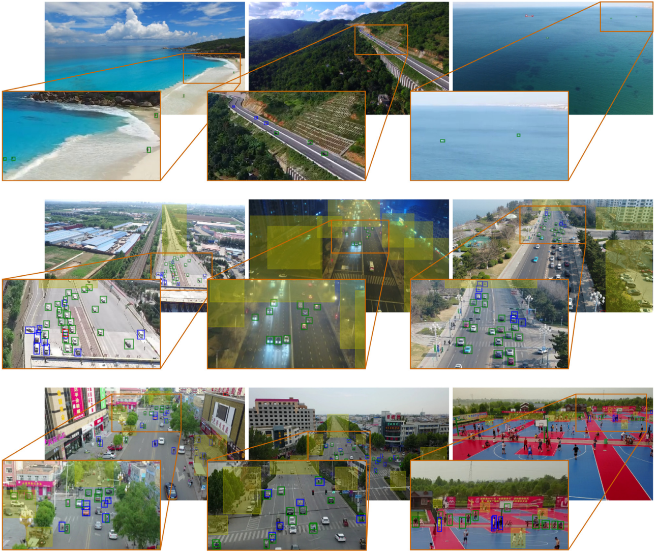
Fig. 7. Some object detection results of STDnet-ST++ for USC-GRAD-STDdb (top), UAVDT (middle) and VisDrone2019-VID (bottom) test sets. A confidence threshold of 0.6 was used to display these images. For each image, green boxes are true positives, red boxes false positives and blue boxes false negatives. The yellow rectangles are ignored regions. Only objects that belong to the XS size are displayed. (For interpretation of the references to color in this figure legend, the reader is referred to the web version of this article.)
