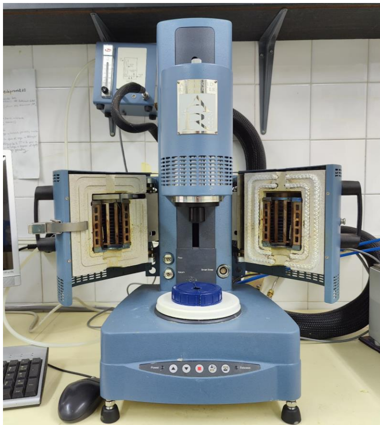
Figure 2.5. Rheometer TA Instruments AR2000.
