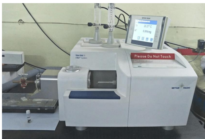
Figure 2.3. TGA/DSC1 Mettler Toledo used in the thermal characterization of this thesis.
