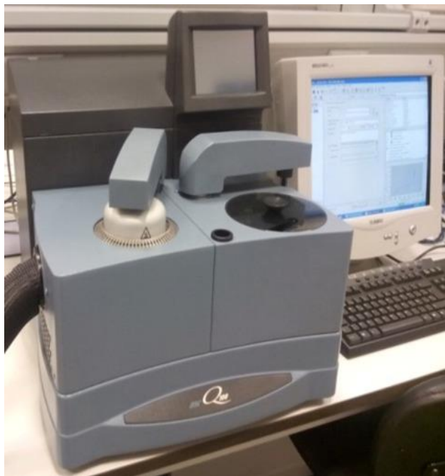
Figure 2.2. DSC Q1000 TA-Instruments used in the thermal characterization of this thesis.
