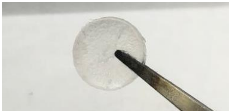
Figure 2.1. Self-standing ionogel synthesised by two precursors silica route.
