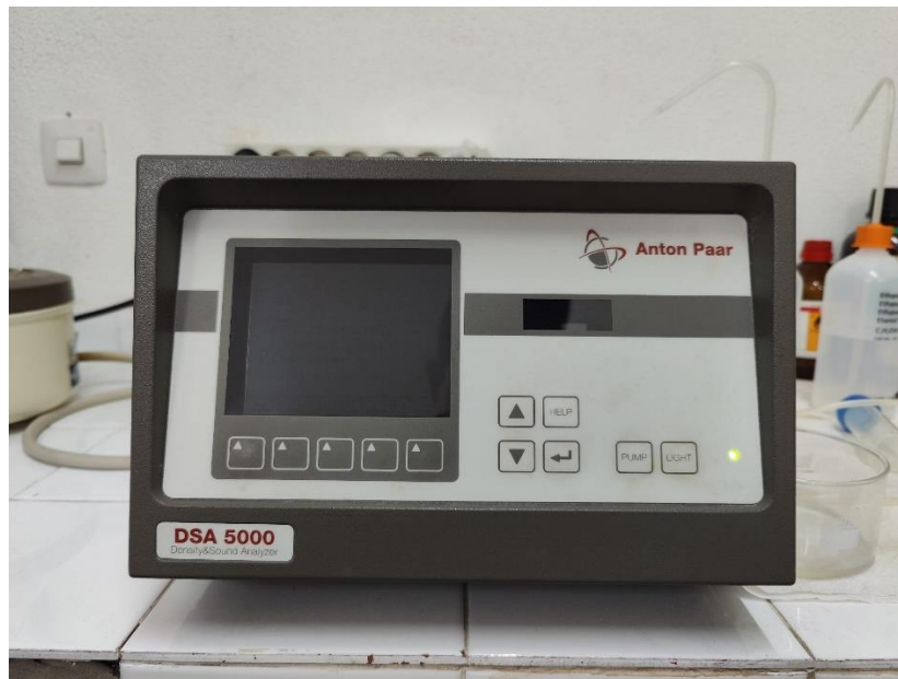
Figure 2.6. DSA 5000 densimeter Anton Paar.
