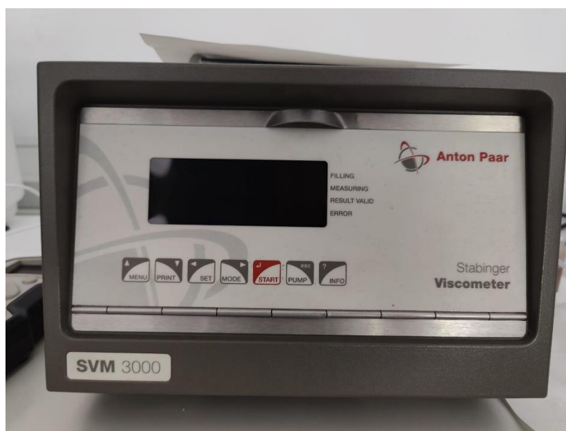
Figure 2.7. Anton Paar Stabinger viscodensimeter SVM3000.
