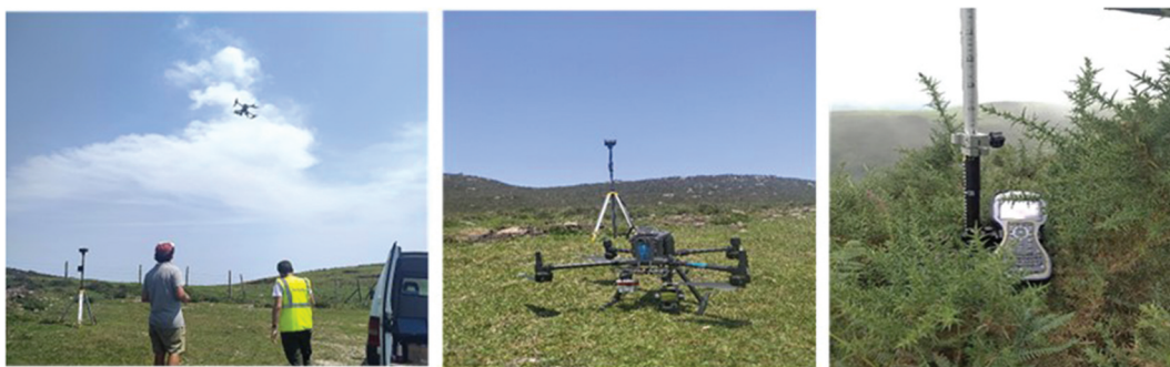
Figure 2. LiDAR and GNSS-RTK equipment used in the study.
