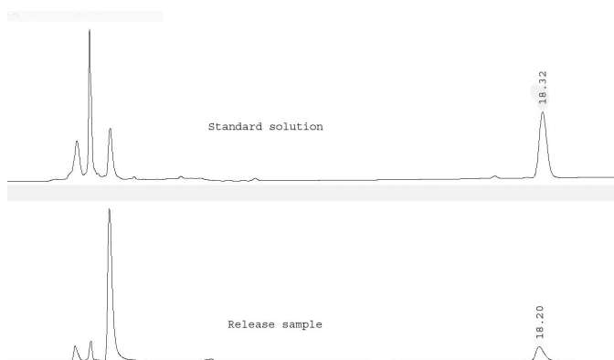
Figure 5: Reverse phase high performance liquid chromatograms of salmon calcitonin (retention time= 18-18.5 min) in a standard buffer solution (top) or after being released from a PEG-coated tripalmitin nanoparticle formulation (bottom).
